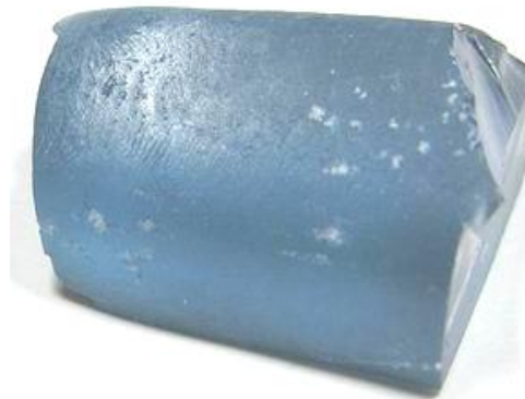
Fig. 2: Faceted and rough flux synthetic spinels. The octahedral crystals have been produced in Russia in the early 90ies. The colour of the blue crystal is due to cobalt. Although not seen this time in the market, blue flux synthetic spinels may also appear again in the trade. © M.S. Krzemnicki, SSEF 2008
