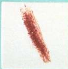
Figure 3.18 Streak of a Mineral Color contrast between hematite mineral specimen and a hematite streak. Massive hematite is opaque, has a metallic luster, and appears black. On a porcelain plate, hematite gives a red streak.
