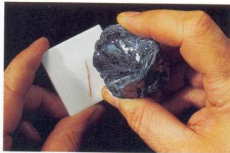
Figure 3.18 Streak of a Mineral Color contrast between hematite mineral specimen and a hematite streak. Massive hematite is opaque, has a metallic luster, and appears black. On a porcelain plate, hematite gives a red streak.
